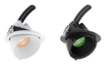
The Mika is a rotatable and tilting LED downlighter that offers a large choice in LED lighting sources and easy interchangeable optics. Create beautiful atmospheres with the ColourFlow technology. The Mika also has a tilt angle of no less than 43°, making it ideal for illuminating objects and walls. It is mains dimmable and has 1-10V, DALI, DMX512 & Casambi Bluetooth dimming options available.
