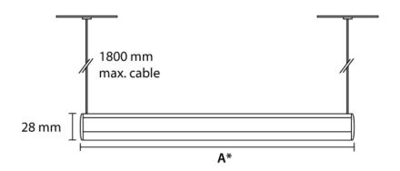
A Model 296 mm Lina Clip RP 30 cm 546 mm Lina Clip RP 55 cm 796 mm Lina Clip RP 80 cm
