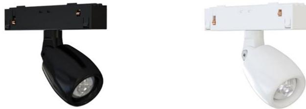
The Focus Compact G3 Track is a 4 watt, ultra-compact zoom fixture that is typically used for showcase lighting solutions in museums, galleries, and shops. The fixture has DMX 512 control and can be dimmed locally with the use of a simple magnet via the CLS Magno Dimming system. The Focus Compact features a stepless zoom range from 13° to 65°.
