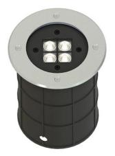
The Revo Compact Inground is a configurable and sustainable lighting fixture. With more than 200 different configurations possible, this fixture can be customized to fit any need. The interchangeable lenses make it easy to change the light setting on the job, and the ventilation gland with Gore-Tex membrane prevents condensation build-up. This fixture is also Future-proof; as all parts are easily interchangeable, the Revo Compact Inground will never be outdated.
