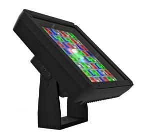
The Quartz is an IP67 outdoor lighting fixture which can be configured in many configurations. It is made from CNC cut, massive aluminium. The ventilation gland with Gore-Tex membrane minimizes the risk of condensation. All electronics fully integrated, no external drivers required.
