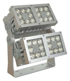
The Revo Basic XXL is an outdoor lighting fixture that offers more than 800 different configurations. It is made from CNC cut, massive aluminium and features an IP67 rating. The bracket construction offers perfect adjustment and alignment, while the ventilation gland with Gore-Tex membrane minimizes the risk of condensation.
