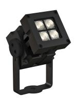
The Revo Compact Basic DMX is a 10 watt, IP67 surface mount fixture that is CNC cut from massive aluminium. Dimming is easy via DMX512. This versatile fixture can be used for façade lighting, gardens, landscape, (art) objects, accent lighting and all other applications where a compact fixture with a surprisingly high light output is required. The sustainable design makes it future-proof; as all parts are easily interchangeable, the Revo Compact DMX will never be outdated.
